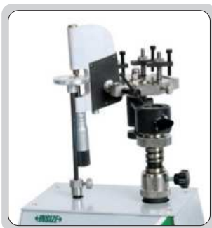
check the measuring force of indicating micrometers
