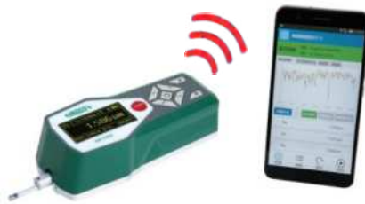
operate roughness tester by mobile phones
