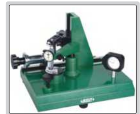
check the effect of lateral force on accuracy of test indicators (half round gauge block is needed)
