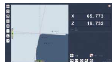
dynamic crosshair automatically adjusting as X and Z axes move, and the cutting tools can be quickly measured through the dynamic crosshair
