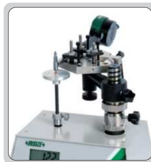
check the measuring force of bore gauges
