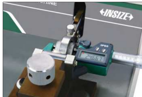
lapping measuring surfaces of outside micrometer
