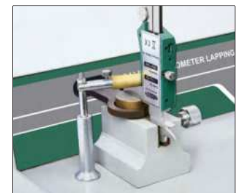
lapping measuring surfaces of caliper lower jaws
