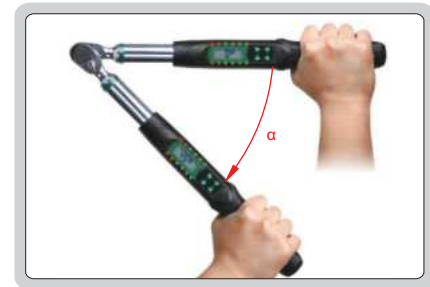
set the desired torque first, after reaching the desired torque, set the angle and turn the wrench at this angle to apply extra torque
