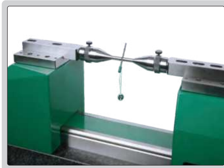
pin gauge measurement
