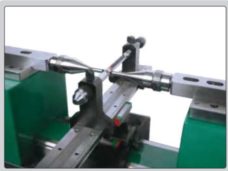
plug gauge measurement
