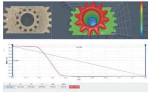
measurement of component bore height
